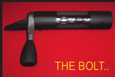
We accurize a wide variety of bolts. Bolts are often reworked with a bushed firing pin to correct firing pin alignment issues and prevent primer cratering. Bolts are also sleeved once the receiver has been reamed to ensure a straight and constant bore diameter. Clearances between the receiver raceway and the sleeved areas of the bolt are typically as low as 0.001" or less.
